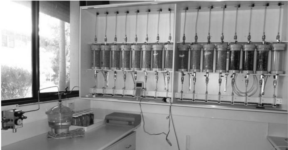
Fig 1- A gas purging flow system was used to treat the insects with constant concentrations of nitrogen and oxygen and maintained low carbon dioxide concentrations during the period of treatment. All 15 cylinders were filled with a known amount (1.8-2 kg) of grain (wheat, barley, oats, lupine and canola).
