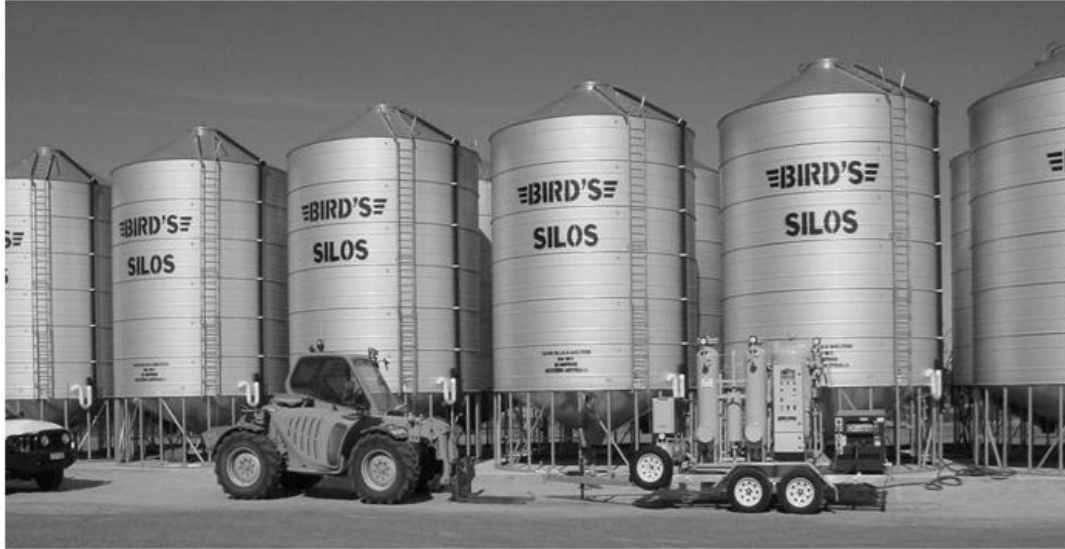
Fig. 2- The farm bin-scale nitrogen application trials were conducted at Doug Clarke's farm near Lake Grace (33.117, 118.607), Western Australia. A pressure swing adsorption (PSA) nitrogen generator (capacity of 30 m 3 of 99.5% N 2 /hour) was used for purging nitrogen to wheat and canola bines (capacity of 75 tonne).
